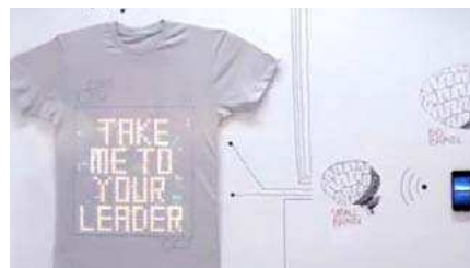
T-SHIRT OS by CuteCircuit. T-shirt with flexible, washable LED screen that can be programmed via a smartphone app to display any image or animation you want. Watch video.
